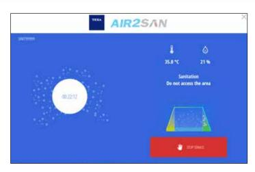
A detail of the IDC5 screen shows the data the operator can monitor in real time: passenger compartment humidity, Ozone level, passenger compartment temperature, time remaining until the end of the sanitation.
